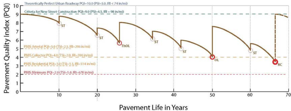
Collector Street on Good Subgrade
