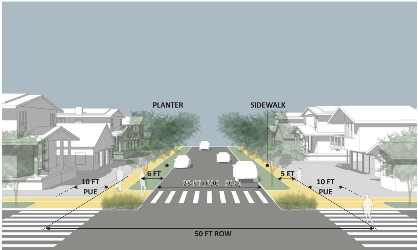
TYPICAL SECTION (Modified YIELD STREET - Envision Taylor Comprehensive Plan) (BUZAN COURT/ NORTH CUTT WAY/ LORETTA LANE)
