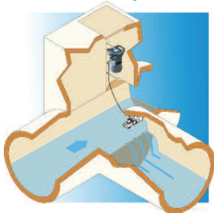
Hach US9001 Down-Looking Ultrasonic Sensor
