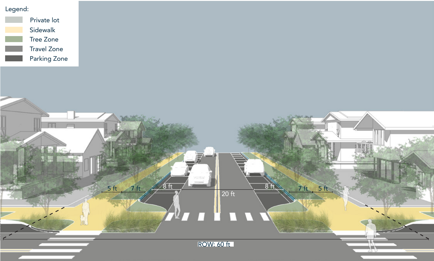
Figure 84: Perspective Section Through Neighborhood Street
