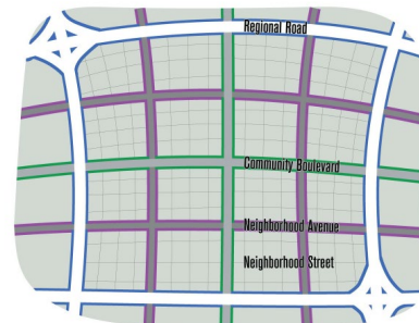
Figure 91: Roadway Hierarchy and Grid Spacing System
