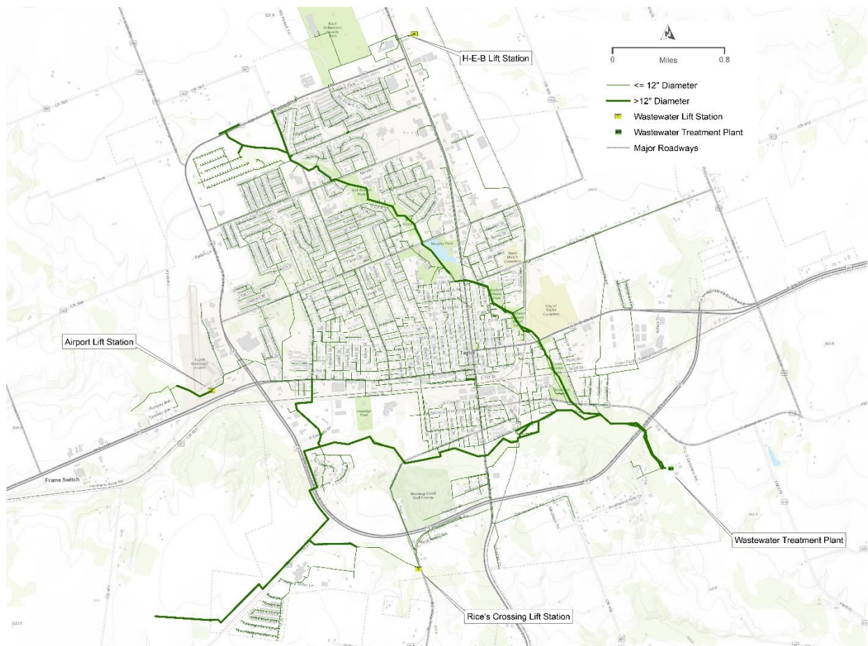
Figure 3-1. Existing Wastewater Collection System
