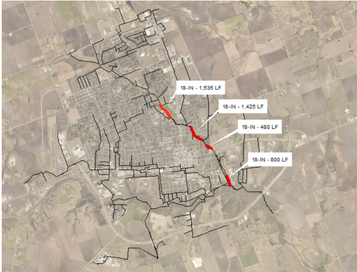
Figure 1. Locations in Current CIP to Upsize Existing Bull Branch Wastewater Interceptor from 15" to 18"
