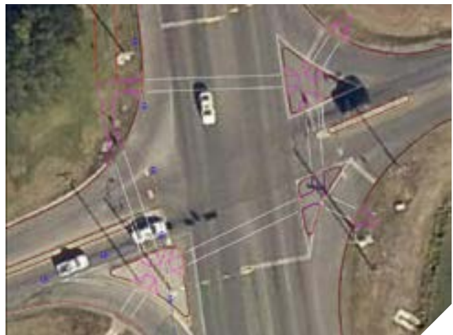
Intersection median and striping improvements at West Lake Drive and SH 95
