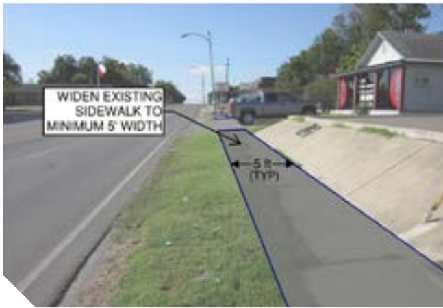
Sidewalk replacement from West 6th Street to West 12th Street
