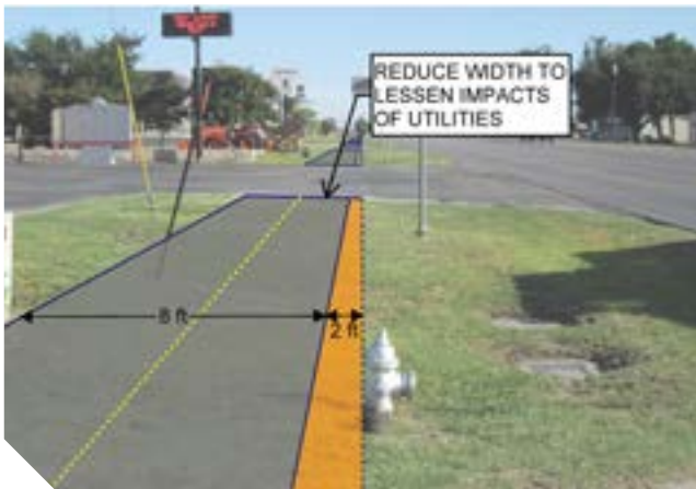
Proposed path modifications to accommodate existing utilities
